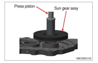
(5) Using the appropriate pliers insert the snap ring and so block the sun gear.
