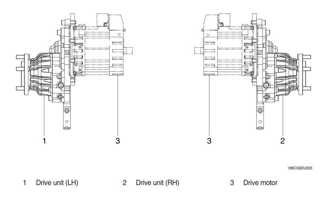
The power of the drive motor which is received from signal of the controller transmits to the drive gear and the power transfered from the drive gear transmits to the drive wheel via the planetary gear and wheel hub. As a result, it is able to drive to forward and reverse of the fork lift.
