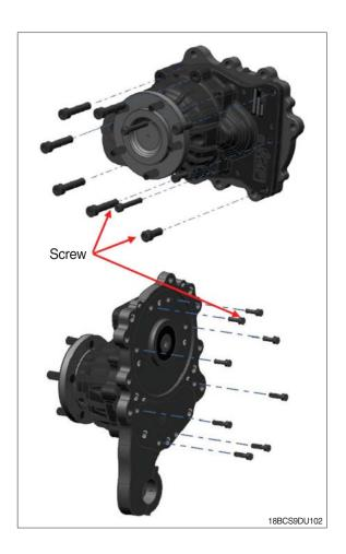
(3) Insert 2 grub screws in the threaded hole extraction of the cover.
