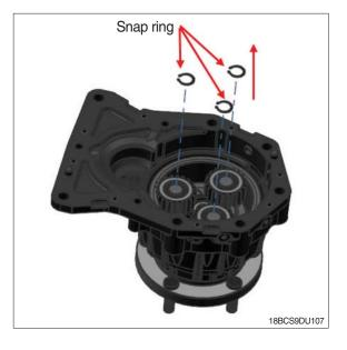
(8) Using the extractor remove the assembled planet gears.
